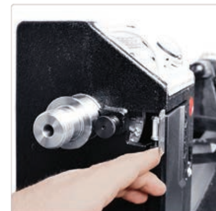
Spindle indexing in 24 points
